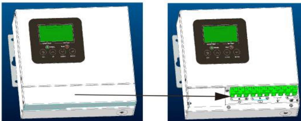
Figure: (Illustration showing how to properly remove the wiring cover)
